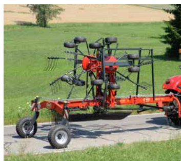
To limit transport height further the tine arms can be removed on the Andex 764. The swath board is folding up automatically.
