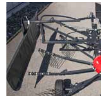
Automatic fold-able swath board with parking stand.
