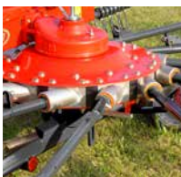
Tine arms can be easily removed.
