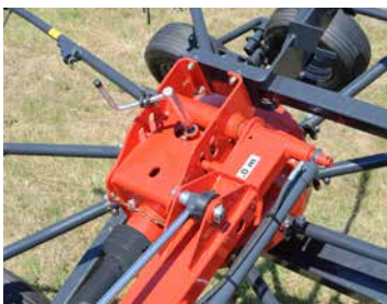
The hydraulic adjustable rotors can be set between 7.00m...
