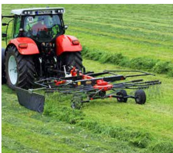
Andex 474T – 4.70m working width and a weight of only 665kg.
