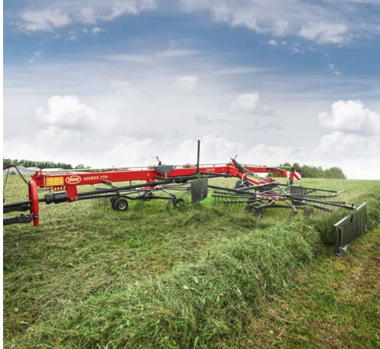
The side delivery concept allows you to collect crop from 15.00m into a single swath.
