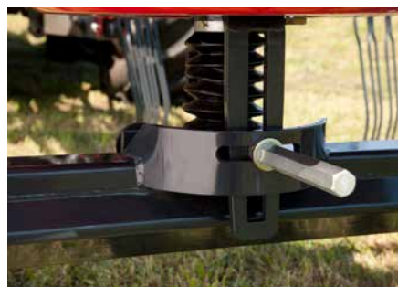
Infinitely variable cam track adjustment allows fine tuning, to obtain optimum raking and swath formation according to crop conditions.
