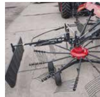
Automatic fold-able swath board with parking stand.
