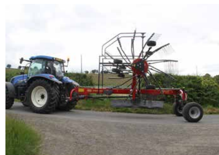
The Andex 804 includes a transport height below 4.00m without leaving the tractor cab and actively steered axles supporting tight turns on headlands and during transport.
