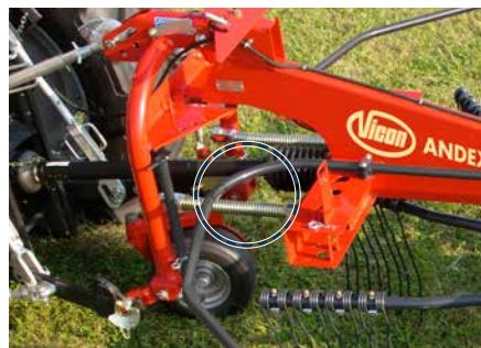
Oscillation dampers ensure excellent running characteristics.
