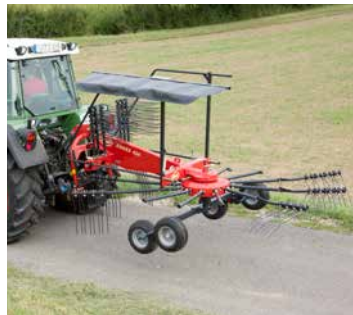
All rakes can be set for reduced transport and storage width by removing the tine arms and placing them on the carrier frame.
