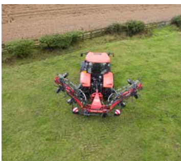
New folding mechanism – ensures even weight distribution during the complete folding sequence.
