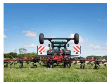
Standard running wheels of Fanex 904C are extra wide 10.0/75 – 15.3 tyres with a generous track width of 2.45m.
