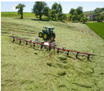
80° turning angle ensures excellent manoeuvrability.
