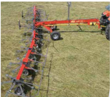
For border tedding the 3 outer rotors are pivoted, to secure evenly inward spreading.
