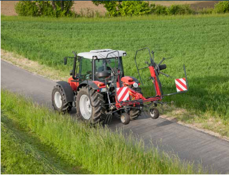
All tedders fold hydraulically from working to transport position and vice versa.
